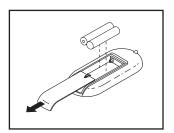
If necessary, remove the old batteries from the remote control. Insert two new "AAA" batteries. **Make sure to insert the batteries as shown in the drawing.** Then, slide the battery cover onto the remote control.
